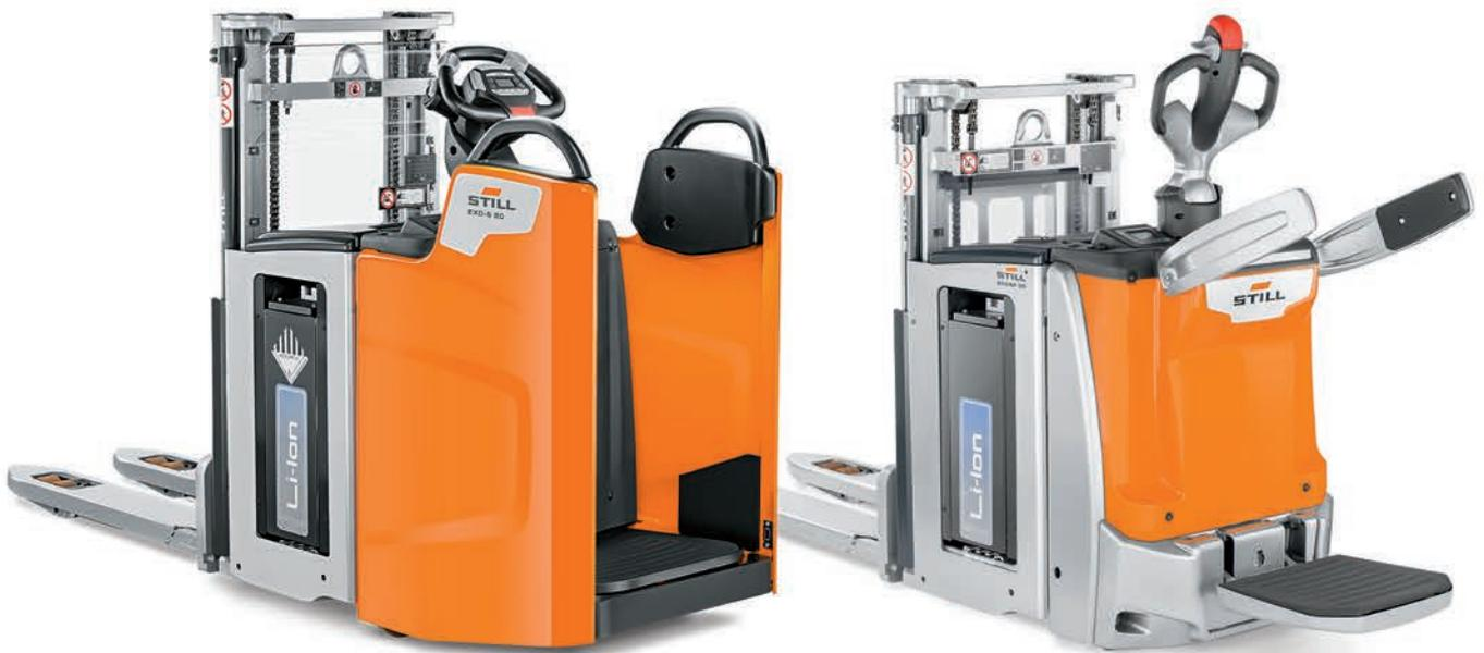
**EXD-SF/EXD-S Double Deck High Lift Pallet Truck with Driver's Stand-on Platform**
