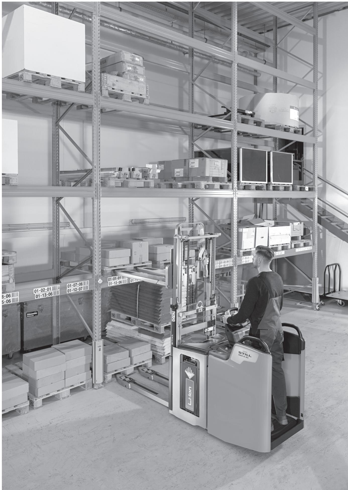
EXD-SF Double Deck High Lift Pallet Truck with Folding Driver's Stand-on Platform
